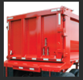
Barn door tailgate with hinges on top and on side
