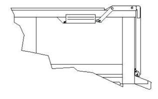
151-3315 Tailgate Hinge Arm Bushing (Long) - 3 Required 151-4300 Combo Hi-Lift Tailgate Cylinder 151-4301 Combo Hi-Lift Tailgate Hinge Arm 151-4302 Combo Hi-Lift Hinge Bushing
