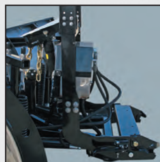
Contoured lift frame for greater ground clearance
