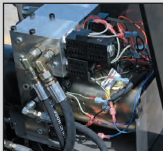
Power unit / hydraulics full size SAE std. cartridge valves, oversized 3/8" rubber hoses, integral valve manifold
