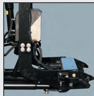
Contoured lift frame for greater ground clearance
