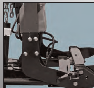
Contoured lift frame provides greater ground clearance
