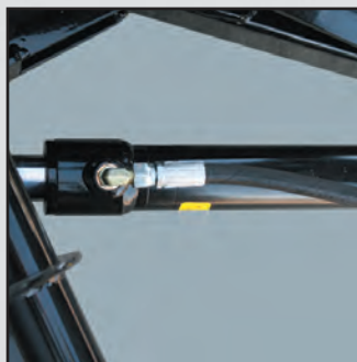
1-1/2" x 12" Double acting angle cylinders allow for real back dragging, standard
