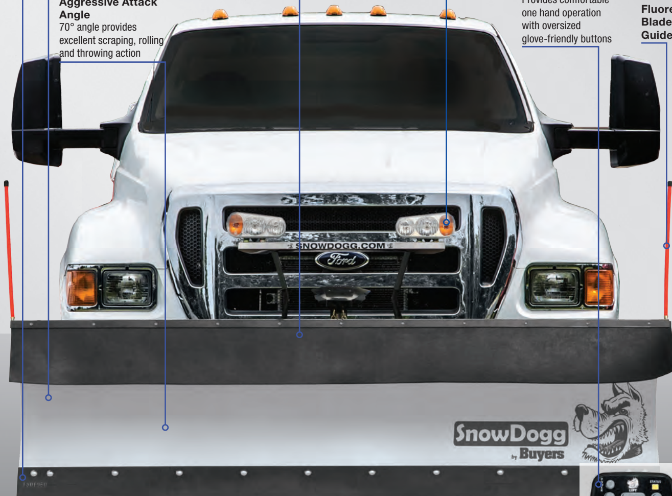
304 stainless steel Tough, corrosion free moldboard is sure to stand up against the elements
