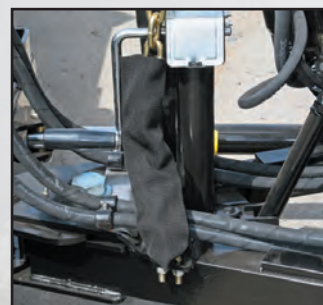
Adjustable/removable jack stand provides maximum flexibility for a wide range of mounting conditions & surfaces
